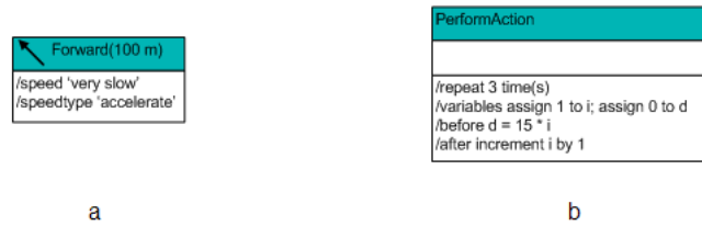
Figure 5.31: Example use of script in graphical notation
