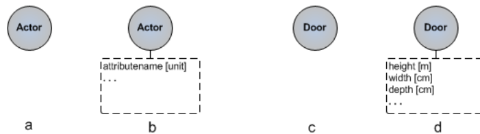
Figure 5.6: Actor (a), detailed actor (b), example (c), detailed example (d)
