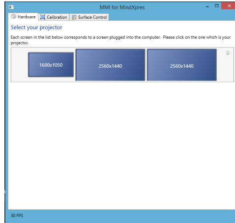
Figure 7-4: Select which detected computer screen is the projector
