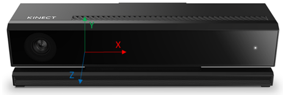
Figure 6-3: Coordinates from Kinect depth sensor.
