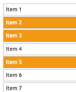
Figure 4.2: Multiple DOM tree elements can be made selectable in jQuery
