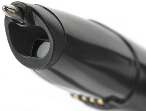
Figure 2.2: The infra-red digital camera in an Anoto digital pen
