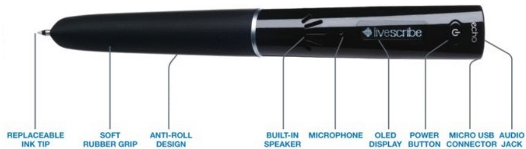
Figure 2.3: Functional overview of the Livescribe Echo Smartpen
