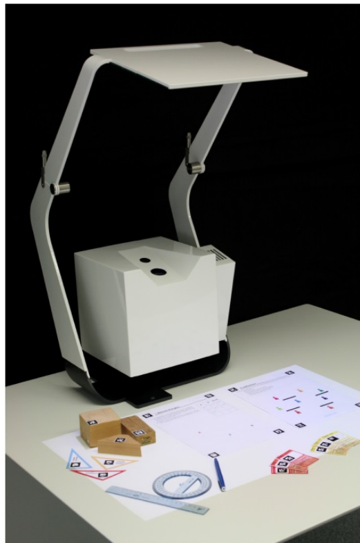
Figure 5.2: The Metroscope, a camera-projector system enabling augmentation on a table
