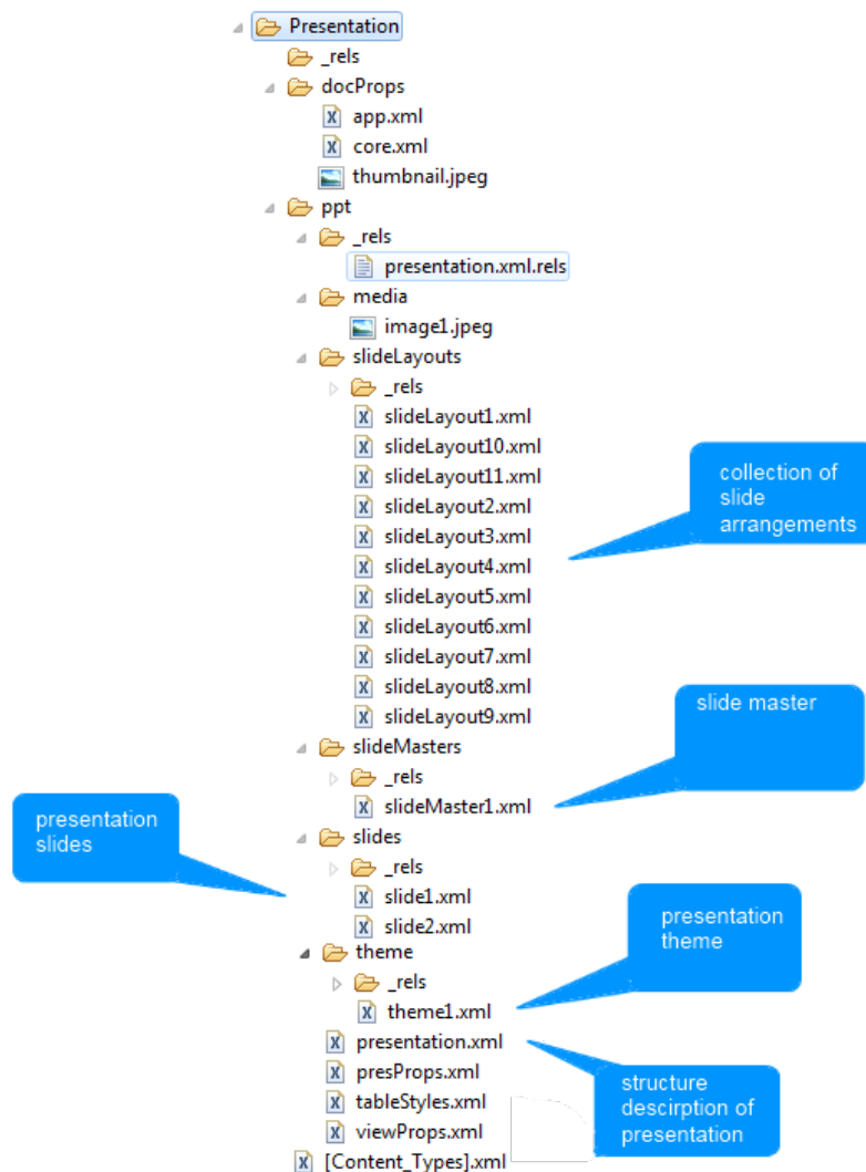
Figure 5.4: Internal structure of a .pptx file
