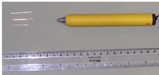
Fig. 5. The co-axial pen with 3 optional nibs (left). Below a ruler provides an indication of scale.
