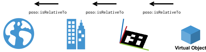
Fig. 3: Relative positioning of virtual objects and markers
