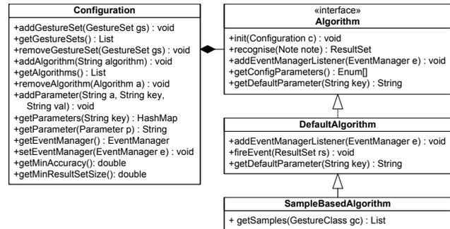
Figure 2. Algorithm class diagram
