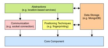
Fig. 1: Component architecture of OpenHPS
