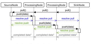
Fig. 3: Pulling data in the process network
