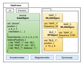
Fig. 4: Data frame containing objects and sensor data
