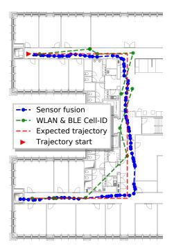
Fig. 8: Test trajectory with WLAN, BLE and IMU data
