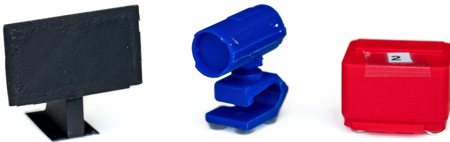
Fig. 9. 3D-printed tangibles (with unique touch point patterns at the bottom) representing a television, a webcam and a printer
