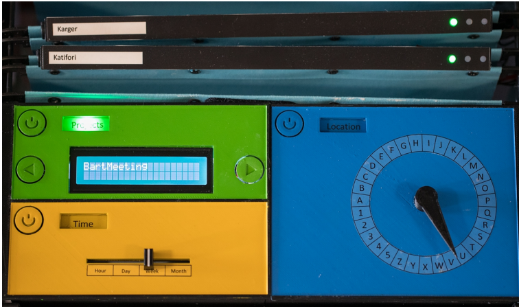
Figure 7.8.: Tangible control panel of the augmented filing cabinet containing three components for exploring contextual, temporal and spatial metadata of the documents
