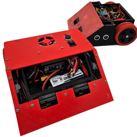
Figure 6.6: Custom-designed Sumo Robot with Wi-Fi connection
