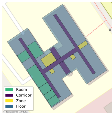
Figure 3.2: GeoJSON representation of a floor with rooms
