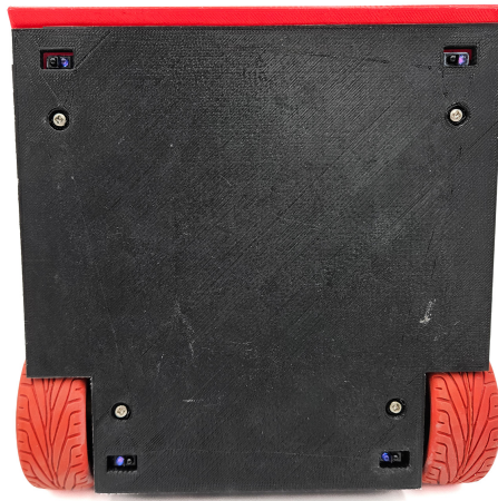
(c) Bottom of the robot showing four line sensors
