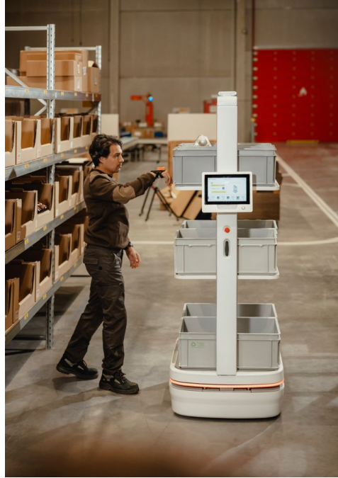
Figure 2.9: Assisted order picking robot from Zeal Robotics
