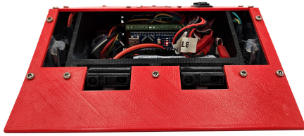
(a) Front of the robot showing two IR distance sensors
