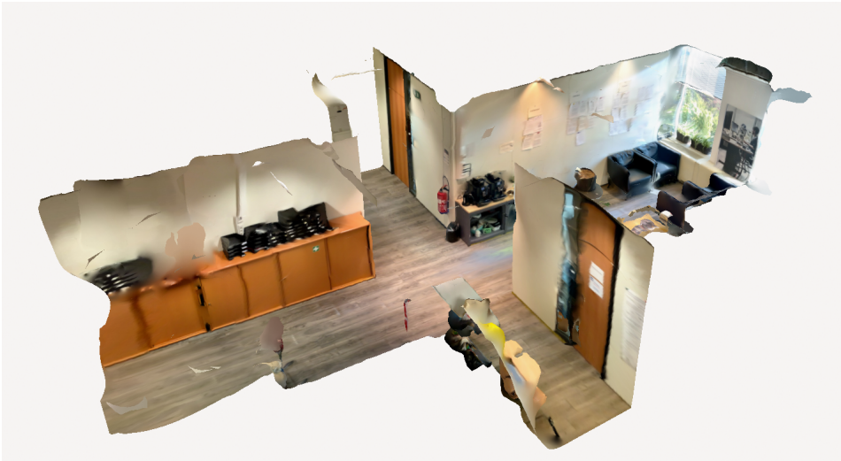
Figure 2.20: Visual SLAM 3D model of a part of the hallway in our office
