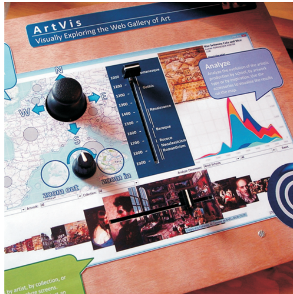
Figure 4.7: The painter's palette contains a small set of phidgets used to control the GUI of the ArtVis system.
