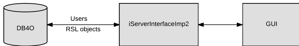
Figure 4.1: Structure of the original application
