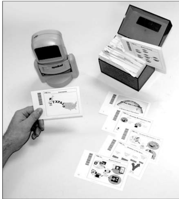
Figure 2.5: The Palette system with presentation cards and scanner [37]
