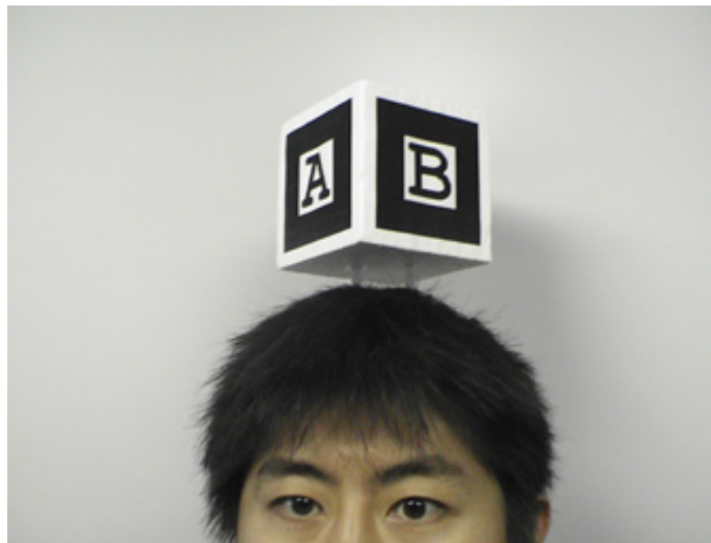
Figure 3.4: The AR toolkit for detecting and tracking the head of the speaker [1].
