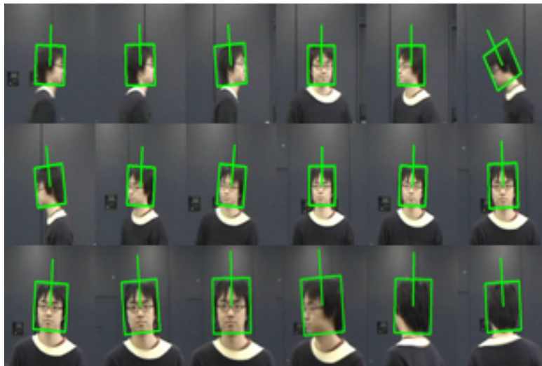
Figure 3.5: The Sub-space and SVR method for tracking the head of the speaker [1].
