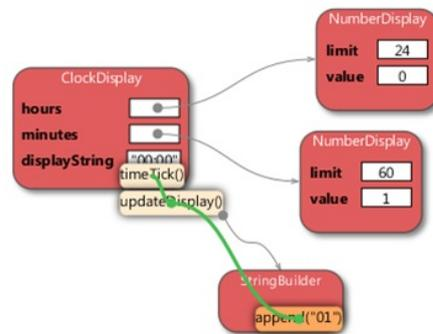
Figure 2-6: An object diagram with overlaid call sequence showing a chain of method invocations [4]
