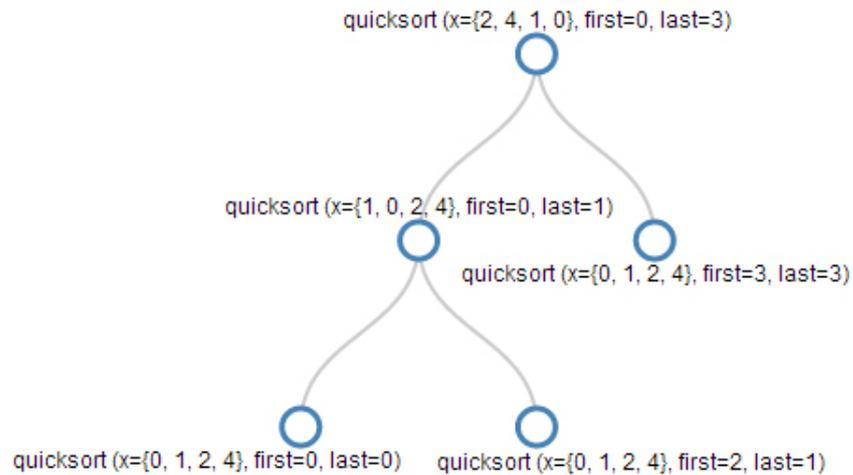
Figure 5-3: A graphical representation of a recursion tree using D3
