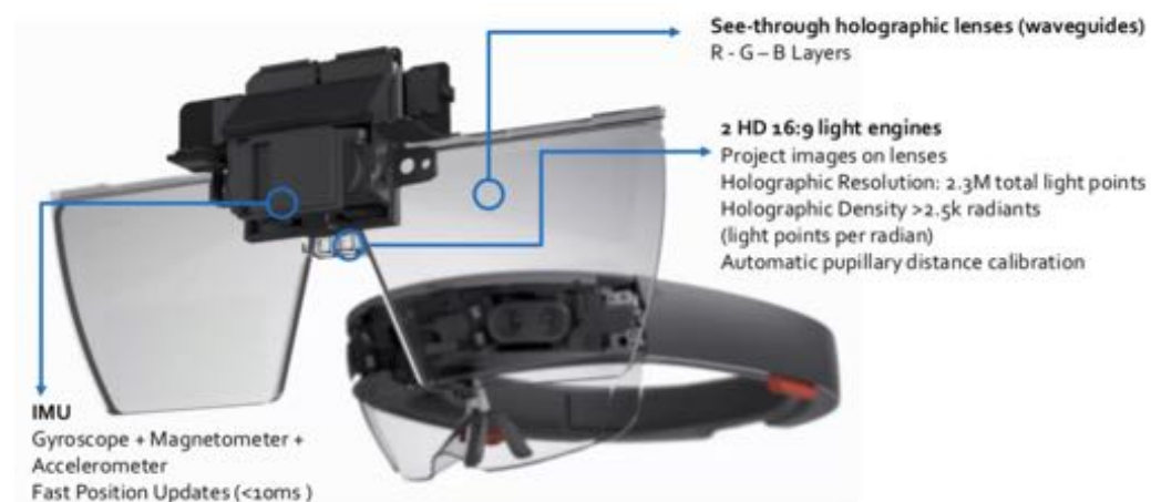
Figure 3.1: HoloLens optics
