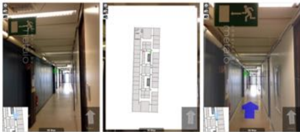
Figure 2.4: Exit icon as AR natural marker for indoor navigation [19]
