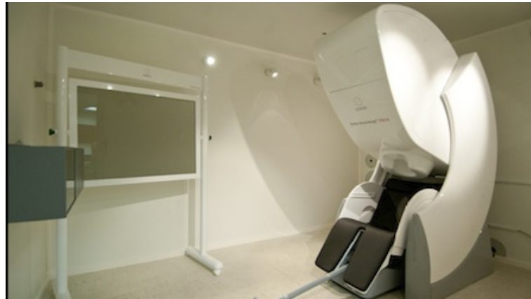
Figure 3.5: A magnetic shielded room with an MEG measuring machine 4
