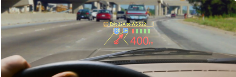
Figure 2.7: Microvision Heads-Up Display, HUDs in vehicles
