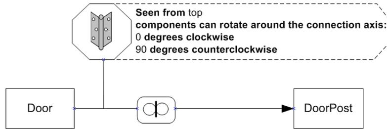
Figure 4.26: hinge constraint example
