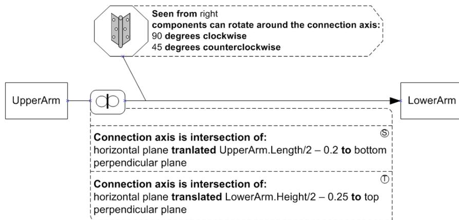
Figure 13.7: Conceptual specification for the UpperArm to LowerArm connection.
