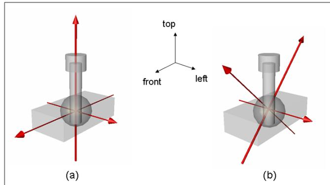
Figure 4.33: possible axes for the joystick constraint
