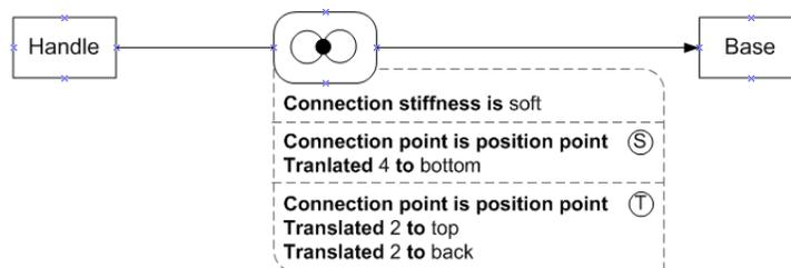
Figure 4.6: connection point relation example
