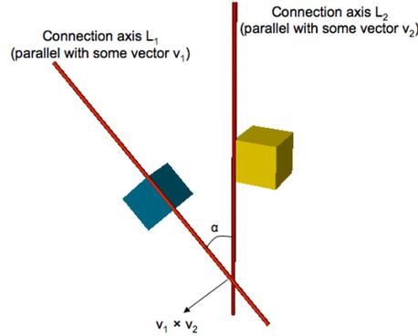
Figure 8.3: Connection axes for source and target may not fall together
