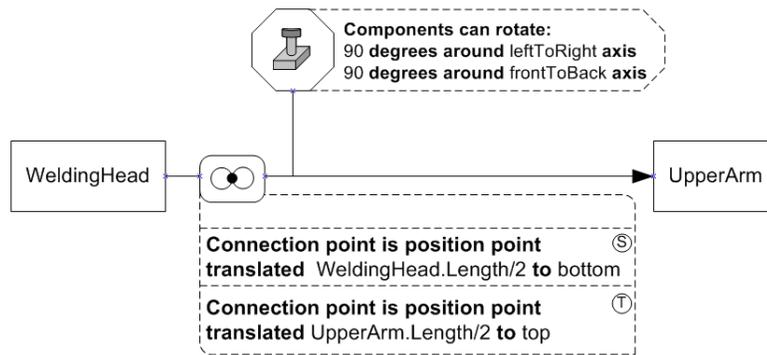
Figure 13.8: Conceptual specification for the WeldingHead to UpperArm connection.
