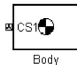
Figure 2.9: Graphical representation of a rigid body in SimMechanics
