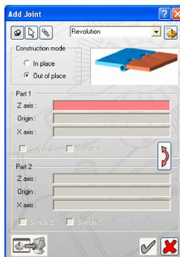
Figure 2.11: GUI for the creation of a revolution joint in MotionWorks
