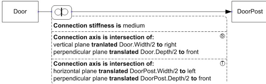
Figure 4.12: connection axis relation example
