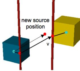
Figure 8.7: Calculation of the translation of the source object
