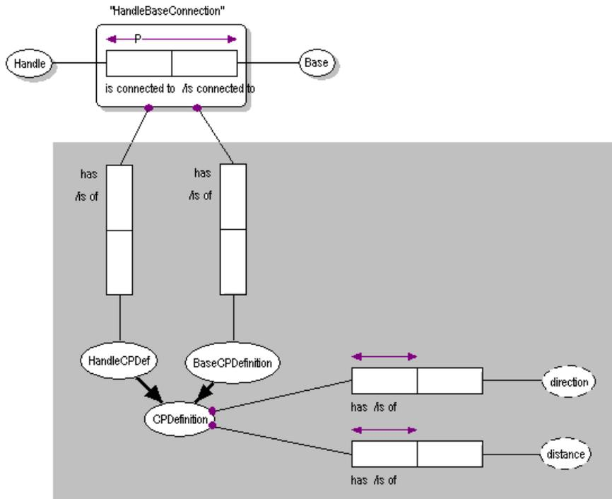
Figure 2.3: Example of the modeling of a connection between two objects using ORM.
