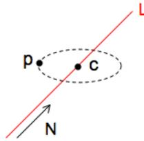
Figure 9.1: Semantics of the hinge constraint
