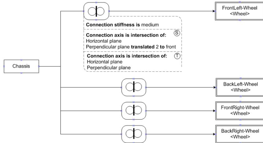
Figure 4.43: Conceptual model for the concept *Car* using roles
