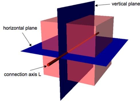
Figure 8.1: Connection axis is the intersection of two planes
