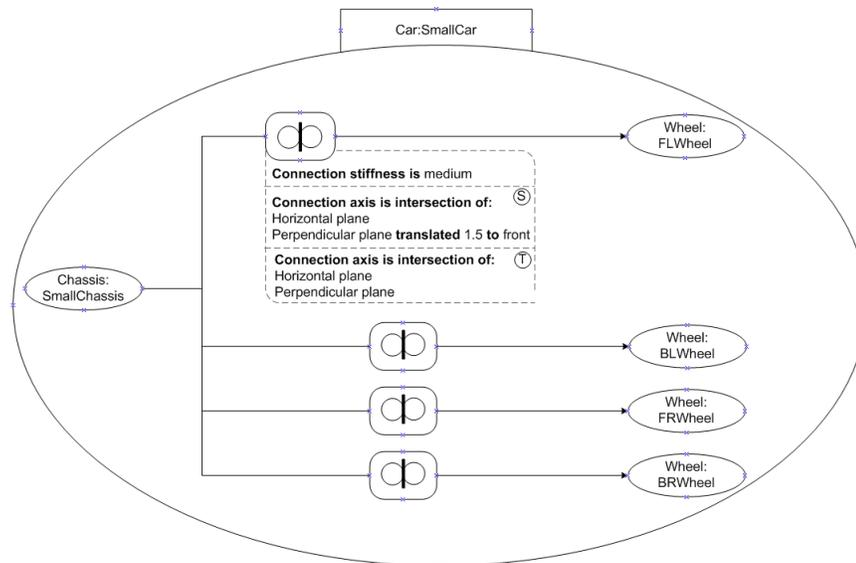
Figure 4.44: `SmallCar` instantiated from the `Car` concept
