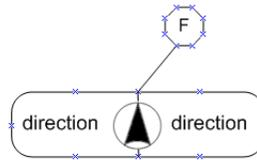
Figure 4.47: graphical notation of the fixed relative orientation constraint
