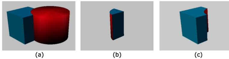
Figure 4.54: CSG operations: (a) union; (b) intersection and (c) difference
