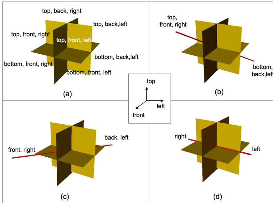
Figure 4.20: possible viewpoint on the connection axis for the specification of a hinge constraint
