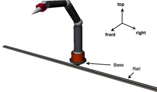
Figure 4.27: Example of a robot arm moving along a rail
