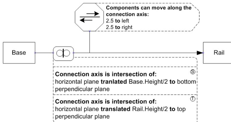
Figure 13.4: Conceptual specification for the Base to Rail connection.
