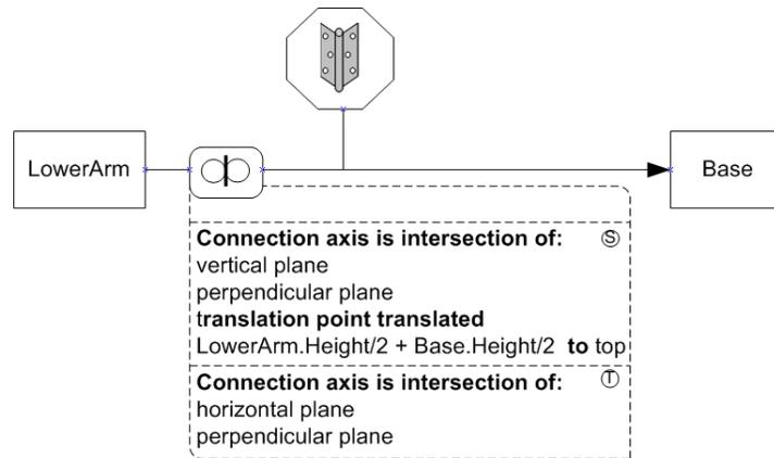
Figure 13.6: Conceptual specification for the LowerArm to Base connection.
