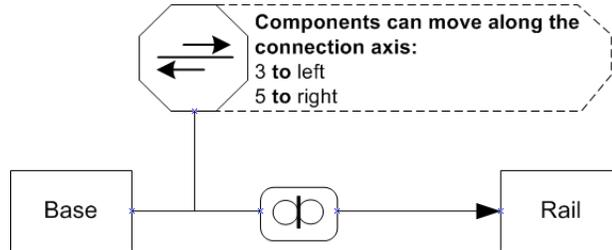
Figure 4.30: slider constraint example
