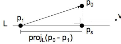
Figure 8.6: Orthogonal projection of a point on a line
