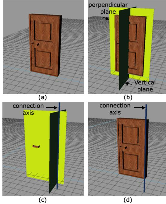
Figure 4.13: Illustration of the connection axis specification for the door object
