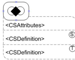
Figure 4.17: Extended graphical notation for the Connection Surface Relation
