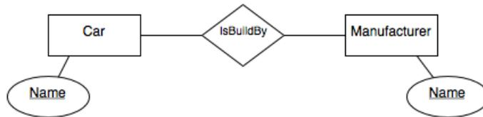
Figure 2.1: Example of an ER model
