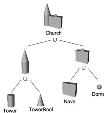
Figure 4.58: An example of a CSG tree
