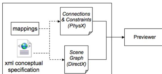
Figure 12.7: Code generation in the Physics Generator Component
