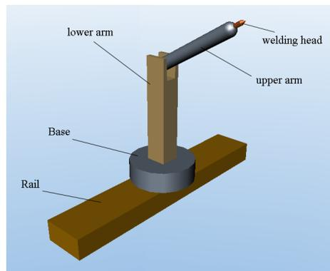
Figure 13.1: The virtual mechanical welding robot
