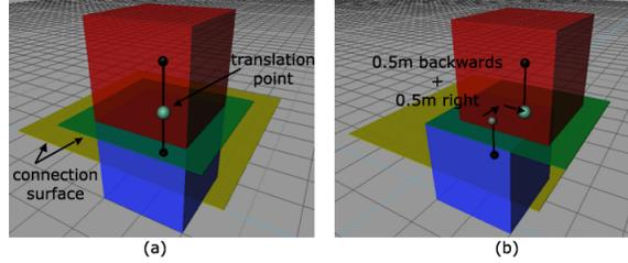
Figure 4.15: translating the translation point in a connection surface relation
