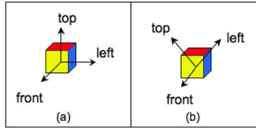
Figure 3.6: (a) default orientation; (b) internal orientation 45 degrees counterclockwise around the front axis
