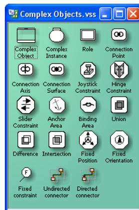
Figure 12.3: Visio stencil for complex object modeling concepts
