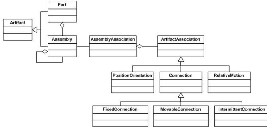
Figure 2.6: Partial class diagram of the Open Assembly Model
