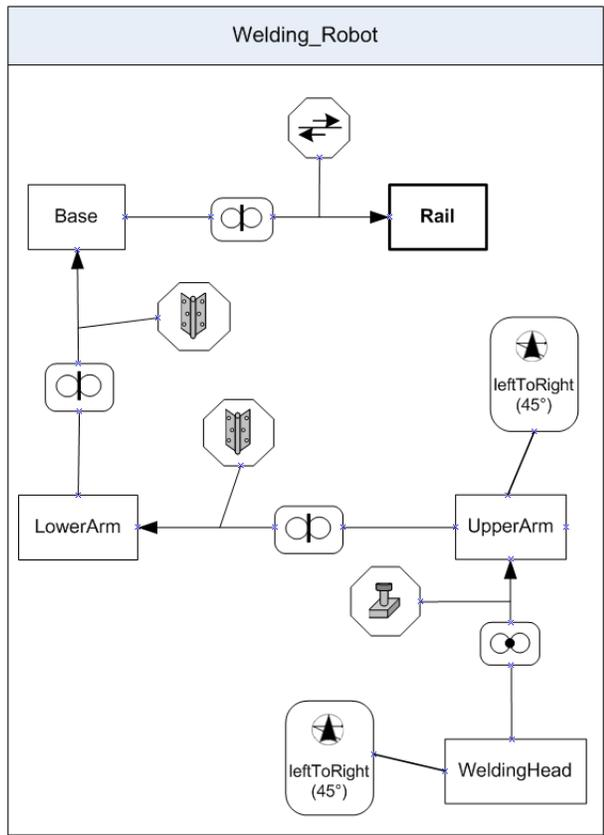
Figure 13.9: Complete conceptual specification for the welding robot
