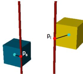
Figure 8.5: Orthogonal projection of source and target position on their connection axes
