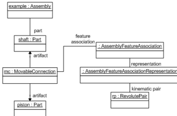
Figure 2.8: Instance diagram of an example assembly in OAM
