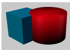
Figure 4.53: Two initial objects used in CSG operations
