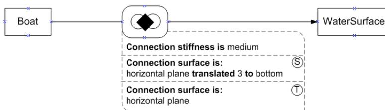
Figure 4.18: connection surface relation example
