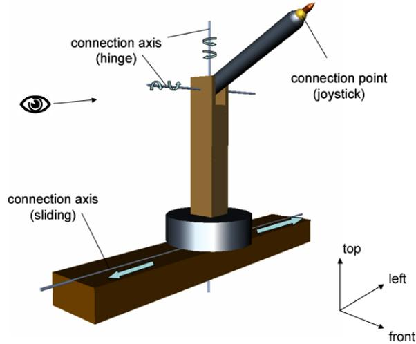
Figure 13.2: Connections between parts of the welding robot.
