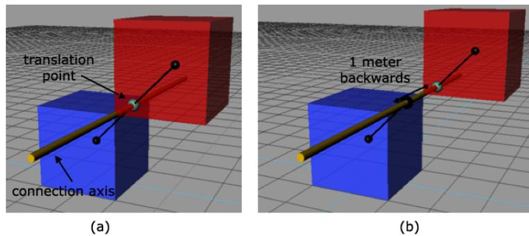
Figure 4.9: translation of the translation point on a connection axis relation
